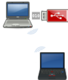
Figure 6: Sample of an offline attack using the covert channel.
