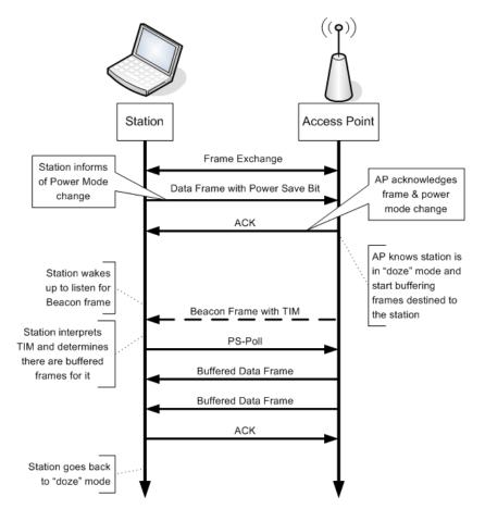
Figure 1: Power Save Time Diagram
