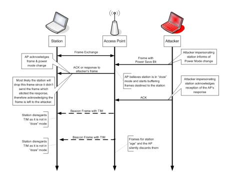
Figure 5: Power Save Denial of Service Time Diagram
