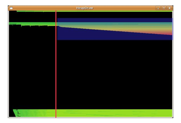
In the picture we can see how the heap evolved during the life of the application dtlogin, while targeting it with an exploit.
