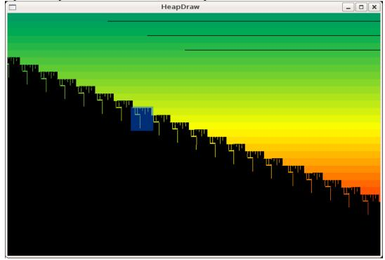
Here we can see how the same patter repeats. We said that the primitive is used several times until the exploit is successful. For every try the exploit need to do several (7) heap operations which compose the basic pattern. In the next picture we zoom in again to see a single try of the pointer-to-code-write primitive:
